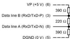
Ends of the Profibus line (bus segment) need to be equipped with terminal resistors, please see the diagram. Terminal resistors may either be part of the connectors or wired to the data card. Termination in the Profibus card is performed by plugging in all three jumpers next to the connector X3
